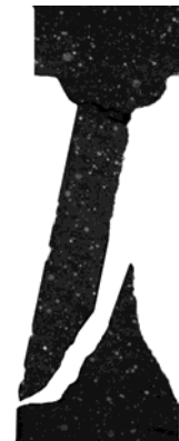
Figure 6. Typical compression failure.
